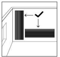
The panels can be mounted vertically or horizontally as desired.
